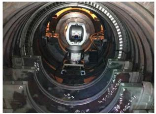
mount the laser tracker at virtually any axially position of a turbine. Using this magnetic bracket on curved surfaces sped up the time needed for setup and reduced the number of moves needed during the measurement process of a turbine, thus increasing accuracy of the readings.
