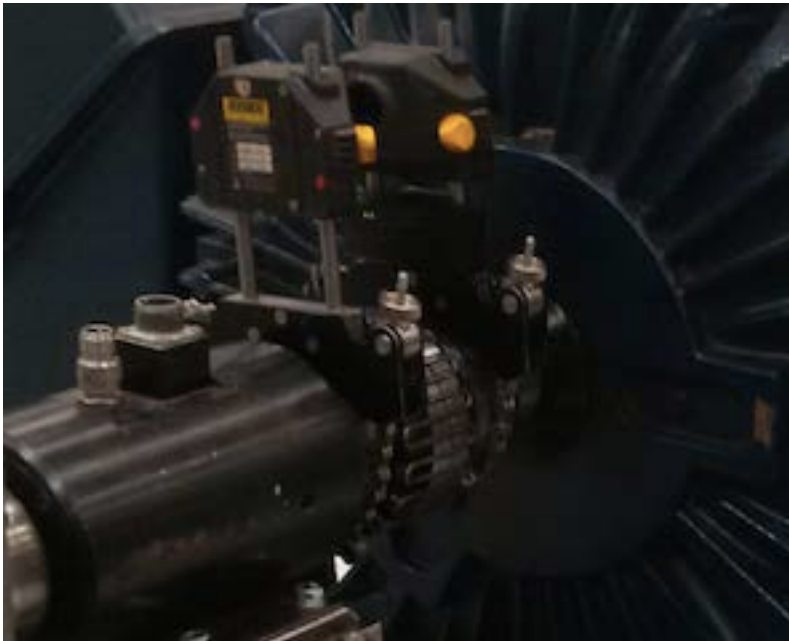
Figure 3. Setup for taking readings between torque cell and electric motor.
