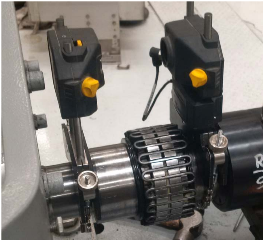
Figure 2. Setup for taking readings between thrust chamber and torque cell.
